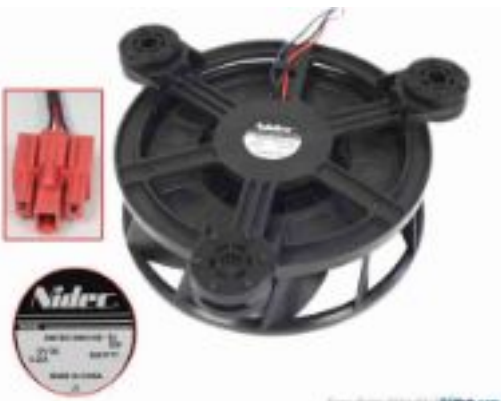
80mm (3.15) INCHES 12VDC 0.15A 0.75W 1800 RPM 1.5mm Nitec.com
